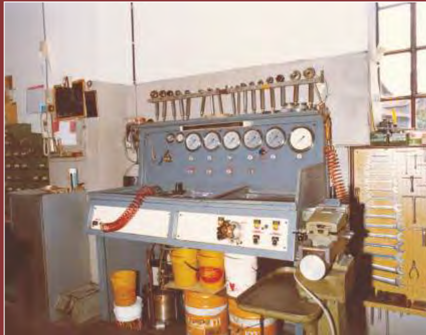
Test bench for hydraulic valve seal
